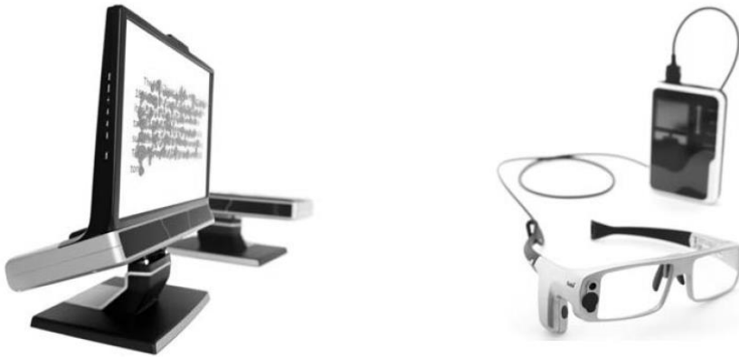
Fig. 1. Stationary eye tracker - Tobii TX300 (on the left) and Tobii Glasses (on the right)
