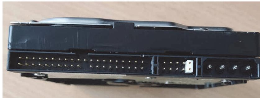
**Figure 2.** A hard drive interface with a jumper on pins. Own study. Photo taken with the POCO X3 Pro.
