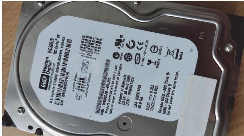
**Figure 1.** A hard drive label (serial number, type of drive, model, capacity, brand, etc.). Own study. Photo taken with the POCO X3 Pro.
