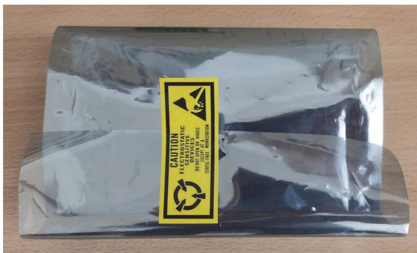
**Figure 3.** An antistatic bag. Own study. Photo taken with the POCO X3 Pro.
