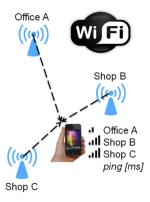
Figure 10. Technologies based on Wi-Fi triangulation. Own elaboration.
