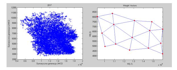
Figure 11. SOM neuron grids generated for the total generations of nJWCD and JWCD for 2017 data. Descriptions: Sumaryczna generacja JWCD (Pol.) - Total JWCD generation (Eng.), Sumaryczna generacja nJWCD (Pol.)- total nJWCD generation (Eng.). Source: Own elaboration in MATLAB and Simulink environment [6, 18, 20, 31].
