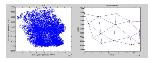
Figure 10. SOM neuron grids generated for the total generations of nJWCD and JWCD for 2016 data. Descriptions: Sumaryczna generacja JWCD (Pol.) - Total JWCD generation (Eng.), Sumaryczna generacja nJWCD (Pol.)- total nJWCD generation (Eng.). Source: Own elaboration in MATLAB and Simulink environment [6, 18, 20, 31].
