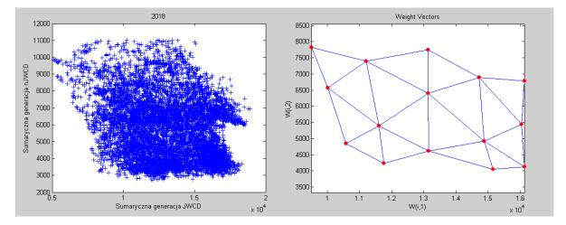
Figure 12. SOM neuron grids generated for the total generations of nJWCD and JWCD for 2018 data. Descriptions: Sumaryczna generacja JWCD (Pol.) - Total JWCD generation (Eng.), Sumaryczna generacja nJWCD (Pol.)- total nJWCD generation (Eng.). Source: Own elaboration in MATLAB and Simulink environment [6, 18, 20, 31].
