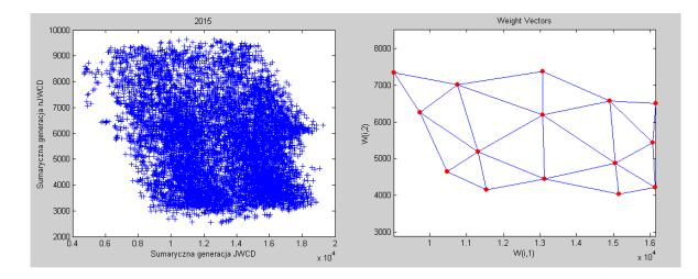
Figure 9. SOM neuron grids generated for the total generations of nJWCD and JWCD for 2015 data. Descriptions: Sumaryczna generacja JWCD (Pol.) - Total JWCD generation (Eng.), Sumaryczna generacja nJWCD (Pol.)- total nJWCD generation (Eng.). Source: Own elaboration in MATLAB and Simulink environment [6, 18, 20, 31].
