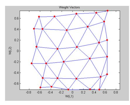
**Figure 2.** Graph visualizing the last step in creating a neuron mesh Markings: W(i, 1) - weight of the X axis, W(i, 2) - weight of the Y axis, Source: Own elaboration in MATLAB and Simulink environment [6, 18, 31].
