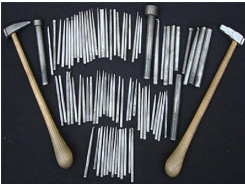
Fig. 9. Various types of hammers and rods for Ghalam Zani (engraving)
